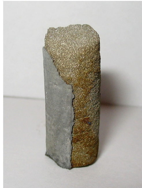
Fig. 5. Photograph of the sample combusted under 48 MPa.
